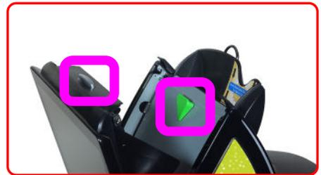
**NOTE:** Instant tickets should never come into contact with this area of the terminal. Latex from the tickets will gum up on the reader and cause failure!
